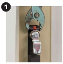
From inside the cabinet, use pliers or vice grips to pinch the snap wedges on both sides of the top. While holding both sides in, work the top of the lock assembly loose by rocking side to side and holding the handle on the front of the cabinet.
